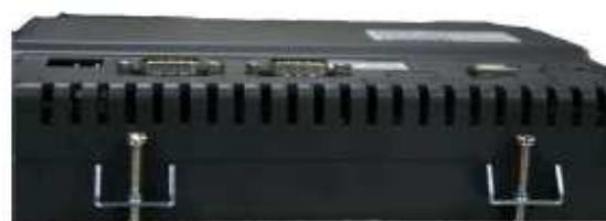
Please secure the screws on the side (the maximum torque for the retaining bracket is 0.3 Nt·m)
